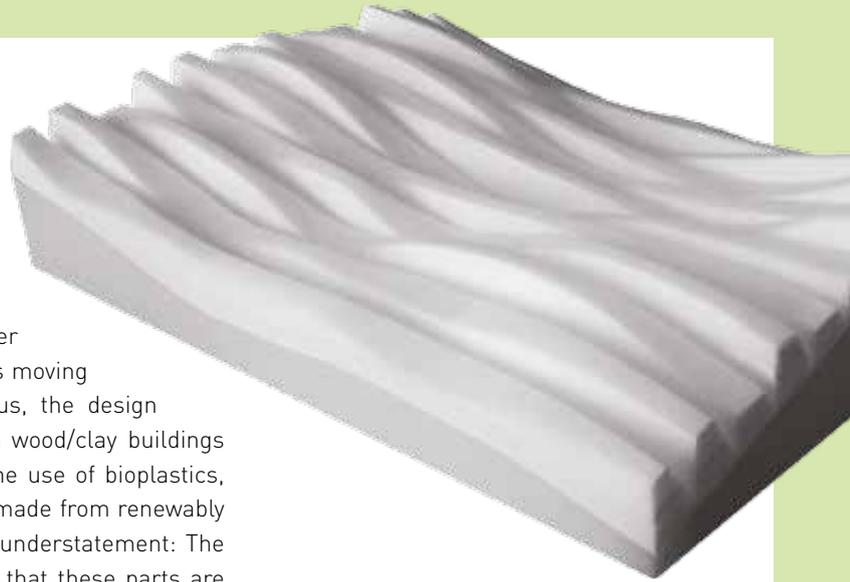
Paneling, thermoformed bioplastic-example by research group: itke, iswa, Tecnaró, Bauer, spek Design (Foto: spek Design)
